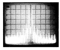
Fig 2—Worst-case spectral display of the FT-990 transmitter during two-tone intermodulation distortion (IMD) testing. Third-order products are approximately 38 dB below PEP output, and fifth-order products are approximately 47 dB down. Vertical divisions are 10 dB; horizontal divisions are 2 kHz. The transceiver was being operated at 100 W PEP output on 3.9 MHz.
