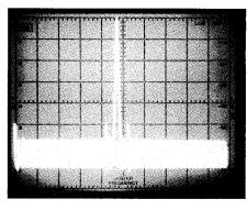
Fig 1—Yaesu FT-990 worst-case spectral display. Horizontal divisions are 500 kHz; vertical divisions are 10 dB. Output power is approximately 100 W at 24.89 MHz. All harmonics and spurious emissions are at least 49 dB below peak fundamental output. The FT-990 complies with current FCC specifications for spectral purity for equipment in this power-output class and frequency range.
